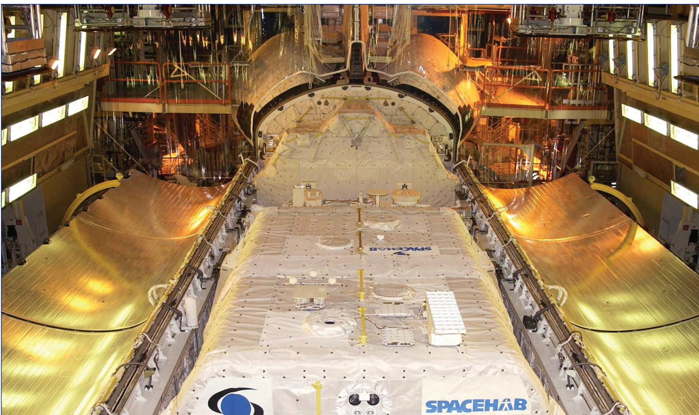
(Below) Columbia's payload bay doors are ready to be closed over the SPACEHAB Research Double Module on June 14, 2002.
